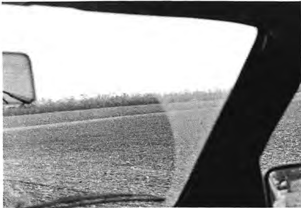
pict.12: Blocked view because of right front windshield column while looking to the right
