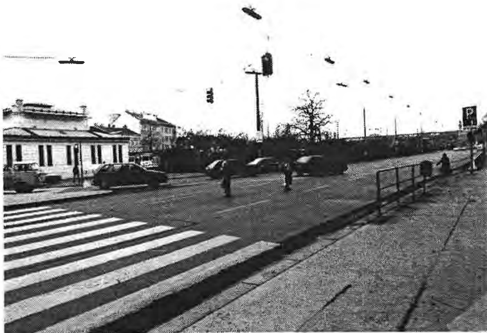
pict.14: Two wide roads meet at a distorted angle, at first unexplainable increased frequency of pedestrian accidents
