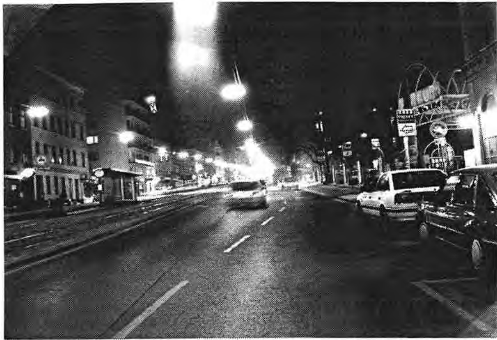
pict.9: Signals which are hanging very closely next to each other are outshined by the streetlights
