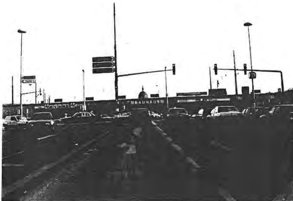
pict.8: The signals for turning left are difficult to perceive in the surplus of objective information
