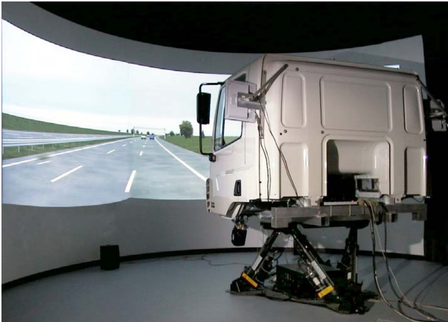
Figure 1: TNO Truck driving simulator (Picture courtesy of TNO Human Factors, Soesterberg, Netherlands)
