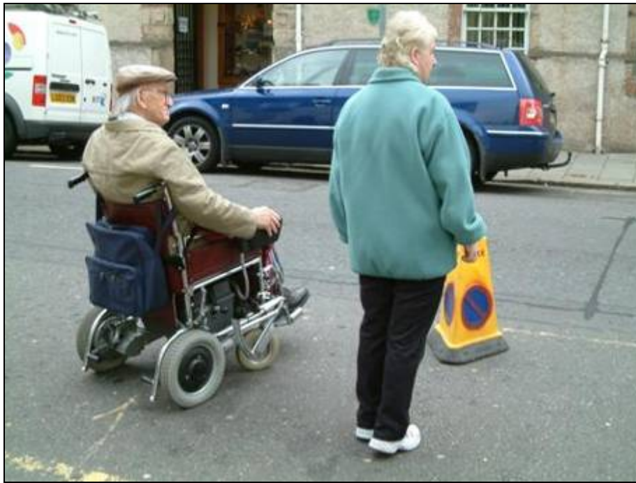
Figure 6: Before. Difficult to cross, poor visibility, no dropped kerbs
