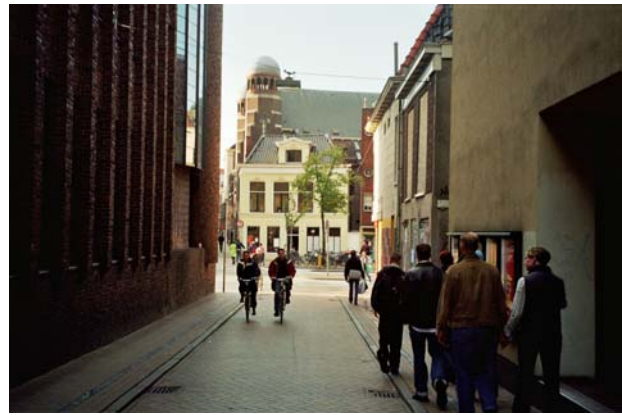
Figure 8/9 Height difference to separate pedestrians from cyclists
