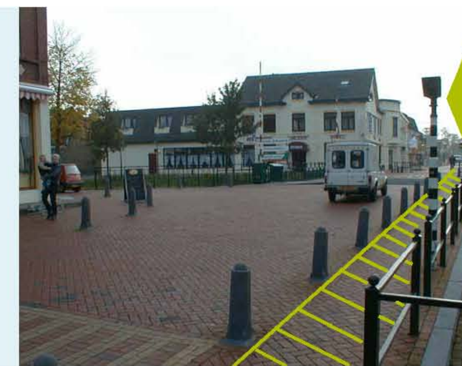
Oosterwolde (NL): A safety zone in a one-level streetscape. But why implementing the poles? A kerb would have been better for guidance and visually less obtrusive.
