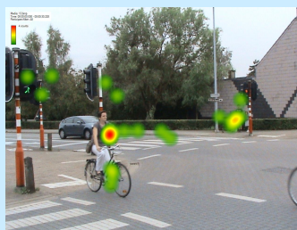
Example of a heatmap: The colors represent the number of fixations (red is high, green is low). The child saw the bicycle and pedestrians, but missed the car
