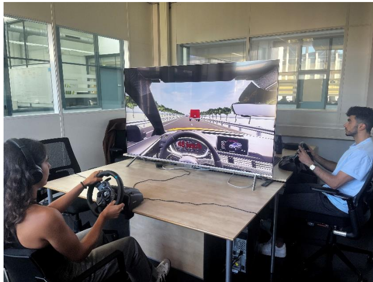
Figure 1: "Reverse Wizard-of-Oz" experimental setup of the driving simulator. During the sessions involving oncoming "human-driven" vehicles, the experimenter (on the right-hand side) pretended to operate an unconnected driving simulator.
