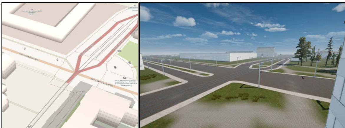
Figure 1: Development process: From the map data (left) to the VR environment (right)
