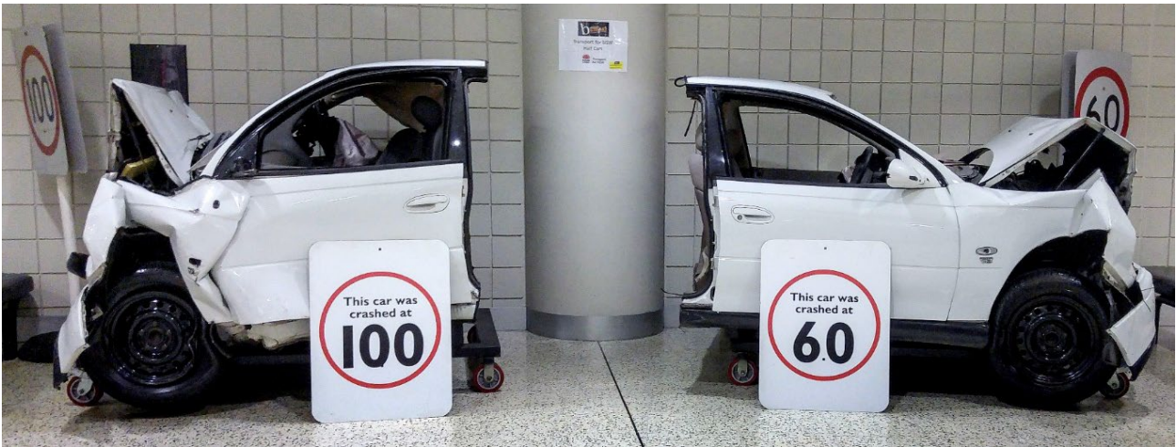
Figure 2.5: Difference in deformation striking a solid object at 60 km/h and 100 km/h
