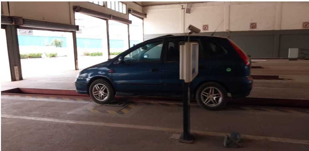
Figure 11: Sideslip and shaker testing for tyres and shock absorbers
