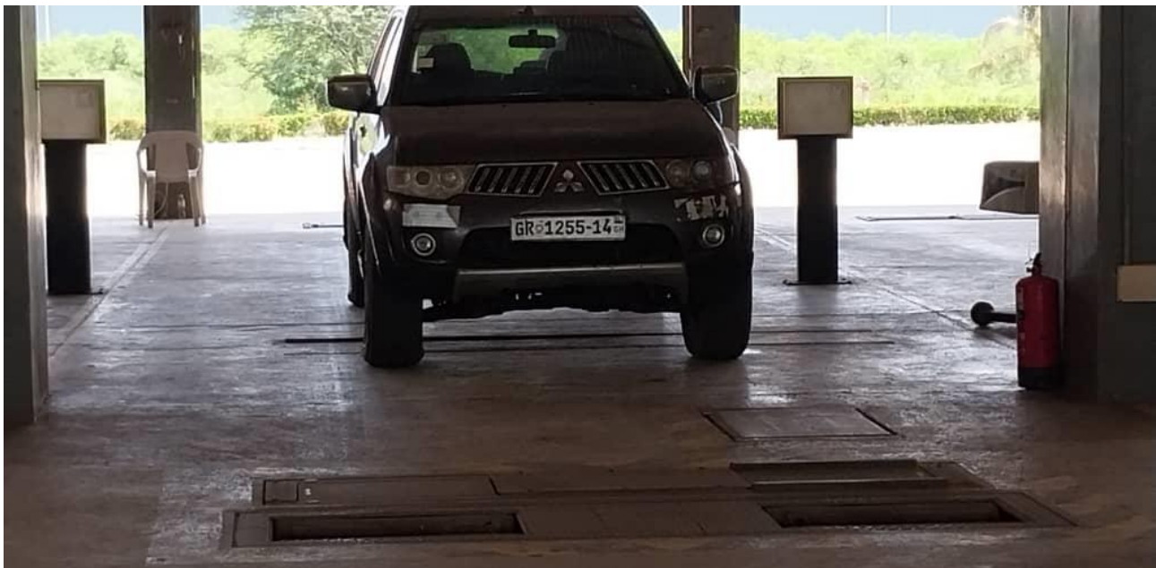
Figure 10: Roller brake testing
