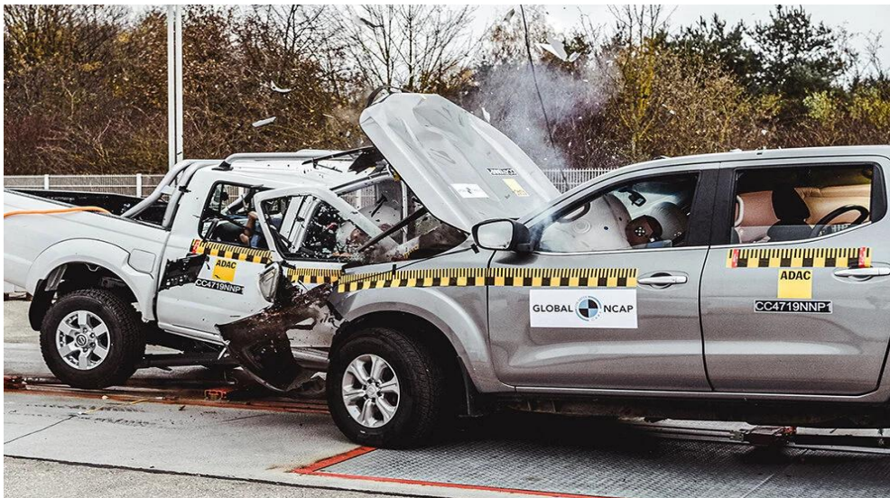
Figure 5: A crash test between a second-hand car (grey) from Europe and a new car made in South Africa (white).
