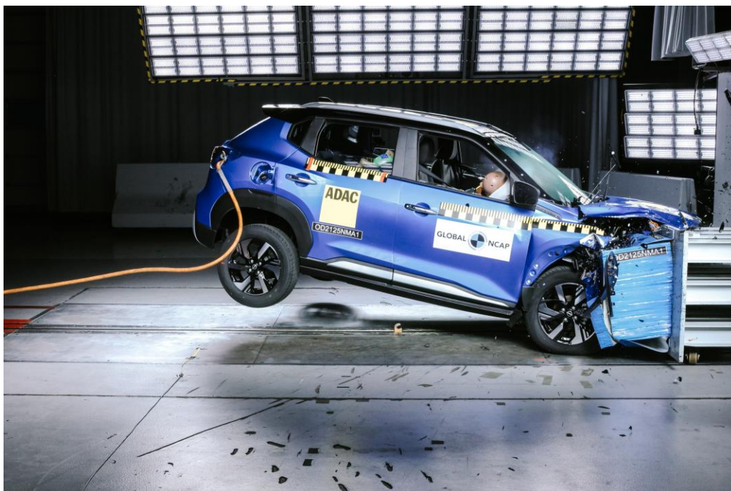
Figure 2: Crash test by Global NCAP for the African market. This car received a 5-star rating.
