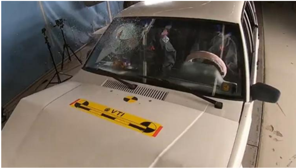
Figure 4: Crash-test video showing an unbelted occupant in a 30 km/h impact.
