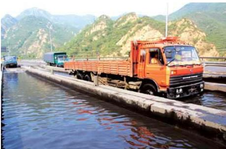
Due to the analysis above, we suggest to set up temperature reducing devices at the top of two long downgrades(K4—K18 and K63—K75)and record the crashes varieties at the same time.
